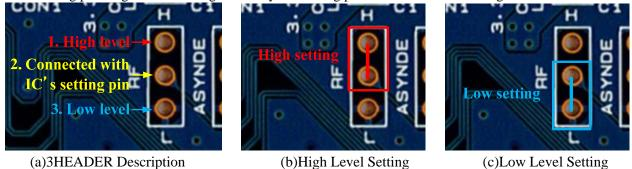
Figure 5 Schematic diagram of High / Low setting description
