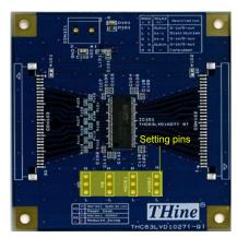
Figure 4 THEVA1027-V2 position of function setting pin
