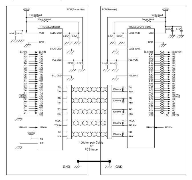
Figure 12. Connection Example with JEIDA Format
