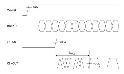
Figure 11. PLL Lock Loop Set Time
