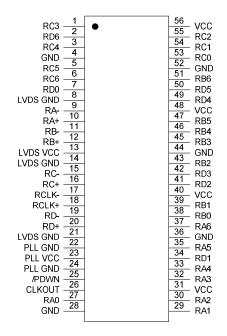
Figure 2. Pin Diagram
