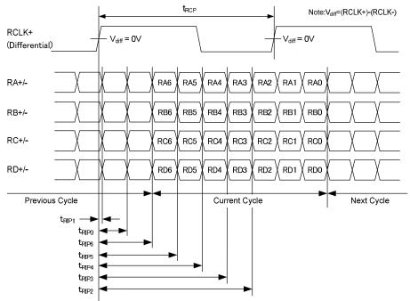
**Figure 7. LVDS Input Data Position**
