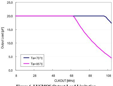
Figure 6. LVCMOS Output Load Limitation
