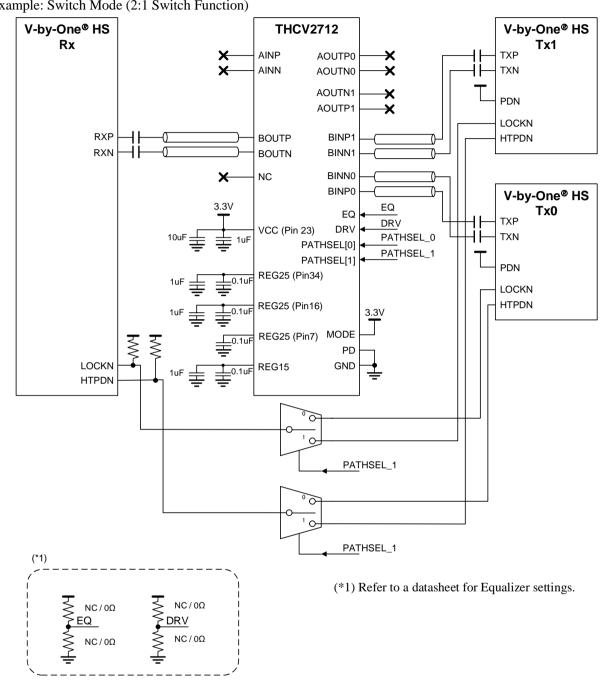
Example: Switch Mode (2:1 Switch Function)
