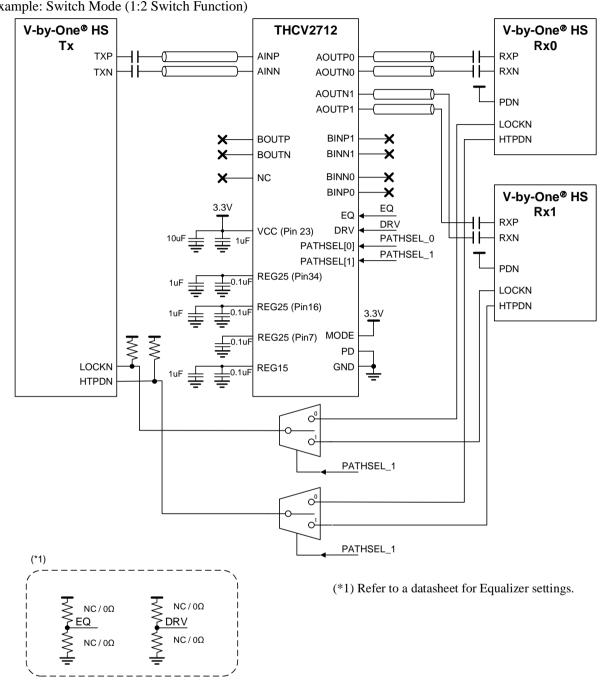
Example: Switch Mode (1:2 Switch Function)
