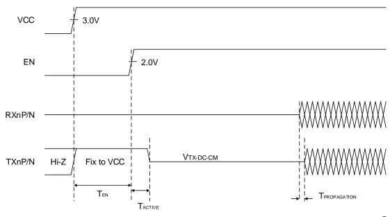
Figure 6. Power on Sequence (SignalDetect Disable/ RxDetect Disable)
