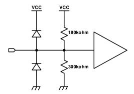
Figure 5. 4-Level LVCMOS Input Schematic Diagram
