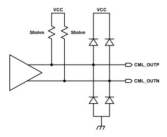
Figure 3. CML Output Schematic Diagram
