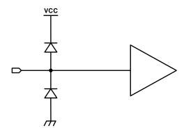
Figure 4. LVCMOS Input Schematic Diagram
