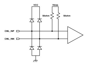
Figure 2. CML Input Schematic Diagram
