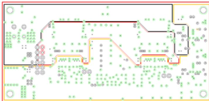
Figure 9-9. Power Plane of THCV216-4LANE
