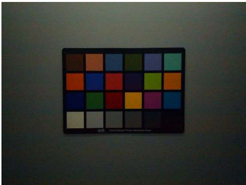
No Low Light Compensation with Fixed Frame Rate
